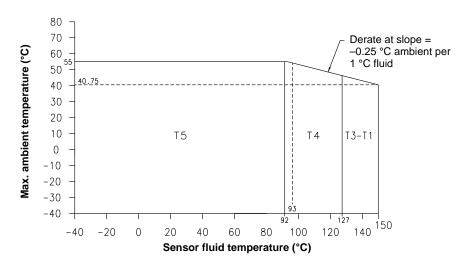
The maximum surface temperature for dust is as follows: T5:T 95°C, T4:T 130°C, T3 to T1:T 153°C.
