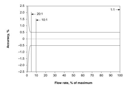
20:1 10:1 1:1 Turndown from maximum flow rate 0.50 Accuracy, ± % 0.50 0.50 Pressure drop 0.1 0.813 54 psi 0.007 0.05 3.4 bar
