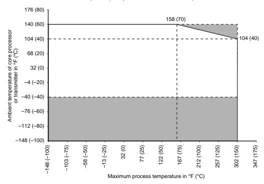
When ambient temperature is below -40 °F (-40 °C), a core processor must be heated to bring its local ambient temperature to between -40 °F (-40 °C) and +140 °F (+60 °C). Long-term storage of electronics at ambient temperatures below -40 °F (-40 °C) is not recommended.
