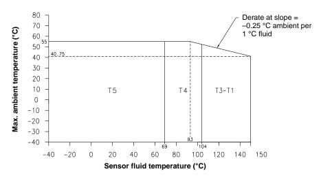
The maximum surface temperature for dust is as follows: T5:T 95°C, T4:T 130°C, T3 to T1:T 176°C.
