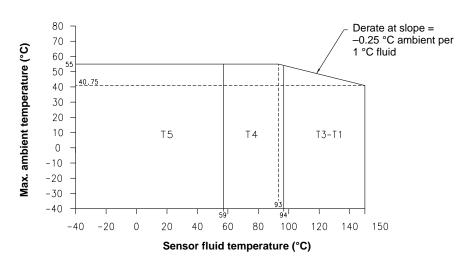
The maximum surface temperature for dust is as follows: T5:T 95°C, T4:T 130°C, T3 to T1:T 186°C.
