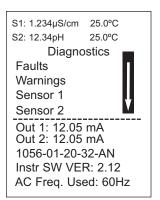
Information about each condition is quickly accessible by pressing the diagnostic button on the keypad. User help screens are displayed for most fault and warning conditions to assist in troubleshooting.
